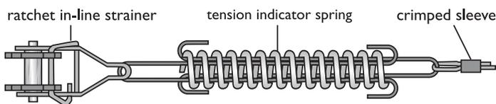
Figure 6. Tension indicator spring used to set and maintain proper high tensile wire tension.
